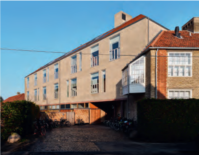
The external walls on both the old and new wings are in yellow brick. The garden wall, which continues into the gate to the new building, is made of recycled brick from the old headteacher’s house – a nice touch and historical gesture.
