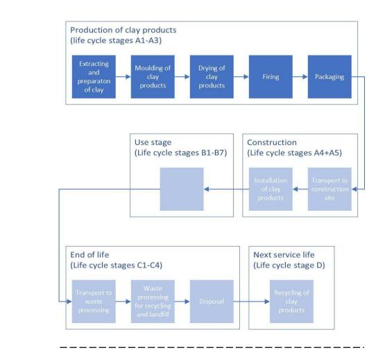
The flow diagram conforms with the requirements in the modular approach and shows the different stages.
